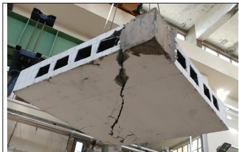
Figure 3.14 : The cracks of the bottom of the voided slab.
