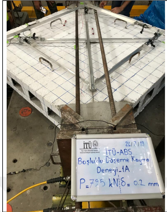
Figure 3.11 : The first crack of the voided slab.
