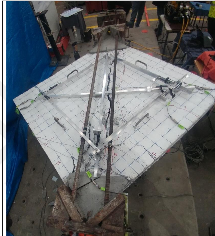
Figure 3.13 : The failure of the voided slab.
