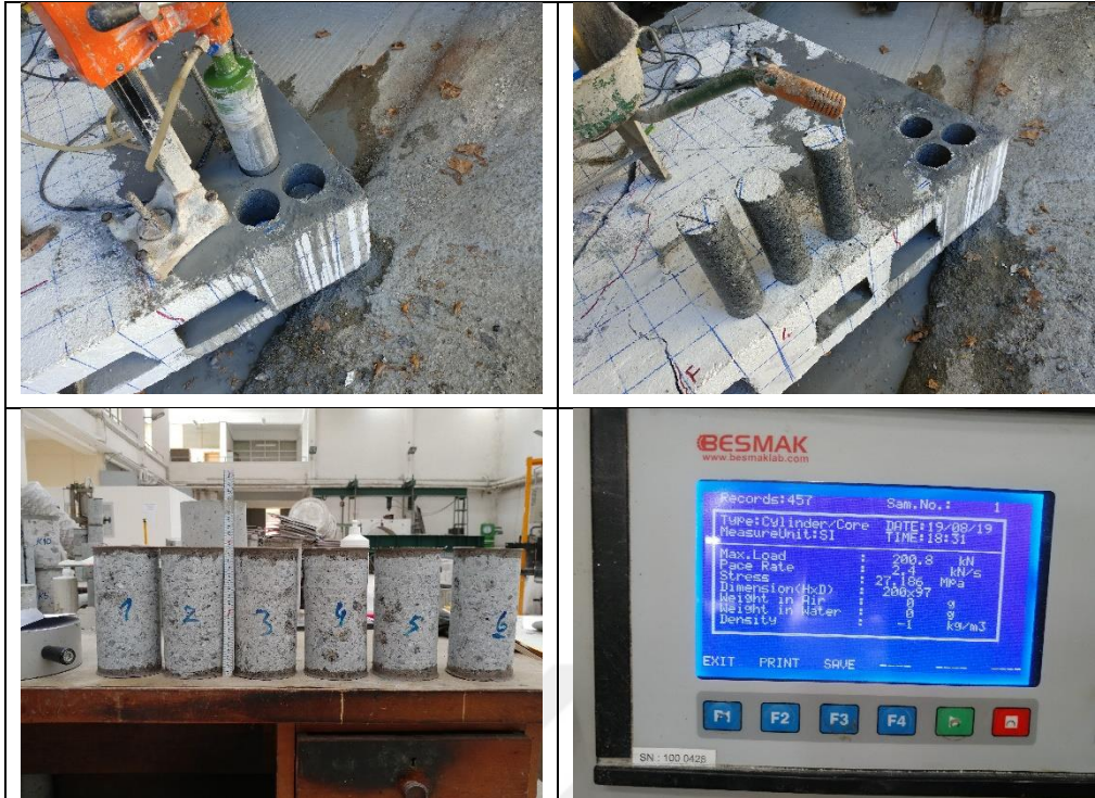
Figure 3.43 : The taken samples for determining the strength of the concrete.
