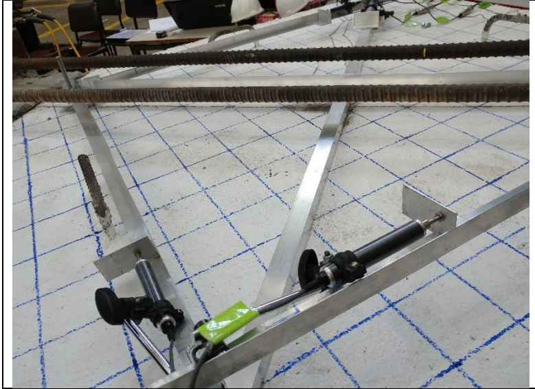
Figure 3.8 : The other two transducers on another corner of the voided slab.
